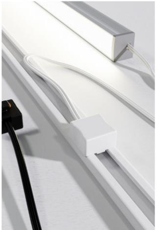
Konnekt **Twist recess-mount** features a slim-line power track made from extruded ABS plastic with integrated copper busbar tracks with an 10-amp rating. It is supplied with push fit ABS end caps. The housing can be bonded or mechanically fixed into a multitude of substrates.
